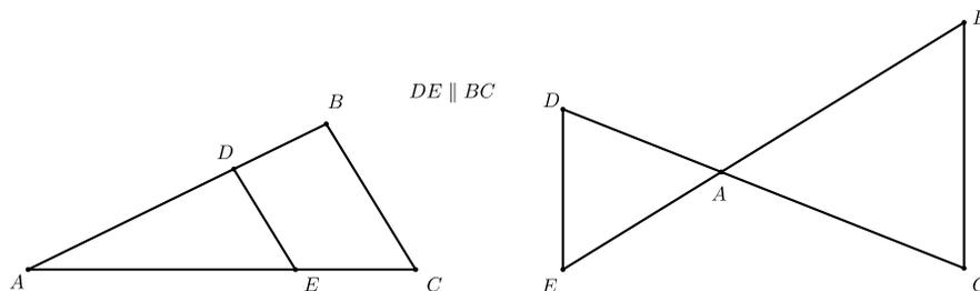
$$\begin{array}{|l} \frac{AD}{AB} = \frac{AE}{AC} = \frac{DE}{BC} \\ \frac{EC}{AE} = \frac{BD}{AD} \\ \frac{AD}{AE} = \frac{AB}{AC} \\ \frac{DE}{AE} = \frac{BC}{AC} \end{array}$$
